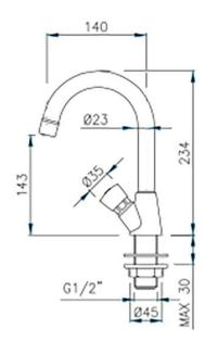
Model TVS9091 is our self closing time flow swan neck basin tap. Non concussive for water saving applications. WRAS approved with a 2 year warranty\*. It is advised that water filters or Y strainers are fitted to the supply pipework to non concussive taps to prevent waterborne debris entering the cartridge (failure to do so will invalidate the warranty if debris has been allowed to enter the tap cartridge)
